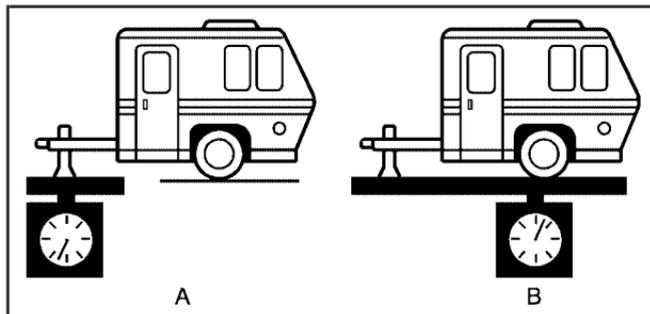
The trailer tongue weight (A) should be 10 percent to 15 percent of the total loaded trailer weight (B), up to a maximum of 400 lbs (181 kg) with a weight carrying hitch. The trailer tongue weight (A) should be 10 percent to 15 percent of the total loaded trailer weight (B), up to a maximum of 1,000 lbs (454 kg) with a weight distributing hitch.
