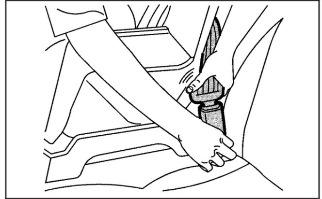
4. Buckle the belt. Make sure the release button is positioned so you would be able to unbuckle the safety belt quickly if you ever had to.
