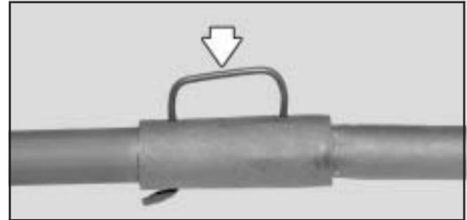
Connect the jack handle (B) and jack handle extension (C) together and press the retention clip (arrow) so it engages.
