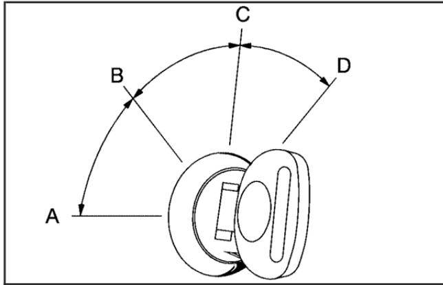
Use the key to turn the ignition switch to four different positions.
