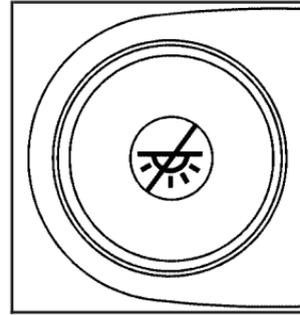
You can use the dome lamp override button, located below the exterior lamp control, to override the automatic operation of the dome lamps.
