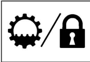
The transmission dipstick is located near the center of the engine compartment and will be labeled with the graphic shown.
