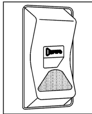
Press the bottom side of the power door lock switch to lock all the doors at once. Press the top side of the power door lock switch to unlock all the doors at once.
