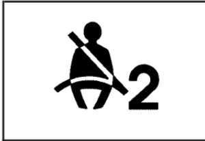
This light and chime reminder will be repeated if the passenger remains unbuckled and the vehicle is in motion.
