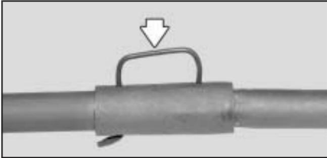
3. Connect the jack handle (C) and jack handle extension (B) together and press the retention clip (arrow) so it engages.
