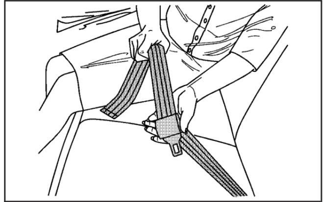
1. Make the belt as long as possible by tilting the latch plate and pulling it along the belt.
