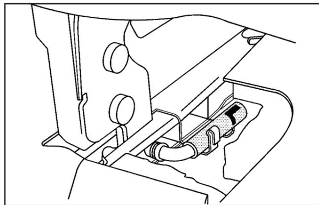
5. Push the pin with the gray cap marked "L" down until it is in the retaining clip.
