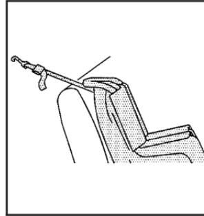
If the position you are using does not have a head restraint and you are using a single tether, route the tether over the seatback.
