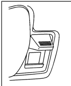
To lock the door from the inside, slide the manual lever on your door down. To unlock the door, slide the manual lever up.
