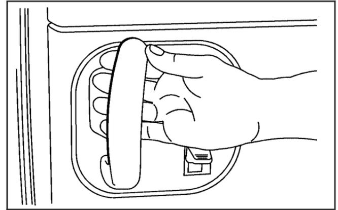
To open the sliding side door from the inside, turn the handle upward and toward the rear of the vehicle. Then, slide the door toward the rear of the vehicle.
