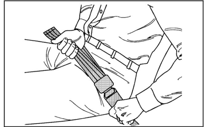
To make the belt shorter, pull its free end as shown until the belt is snug.
