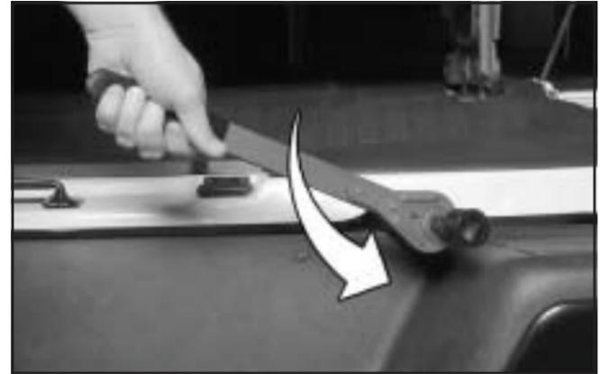
2. Put the flat chisel end of the wheel wrench on an angle through the hole between the body and the bumper. Be sure the flat end connects into the hoist shaft.
