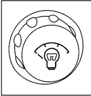
Press this knob located next to the exterior lamps knob to extend it, and then turn it to adjust the instrument panel brightness.
