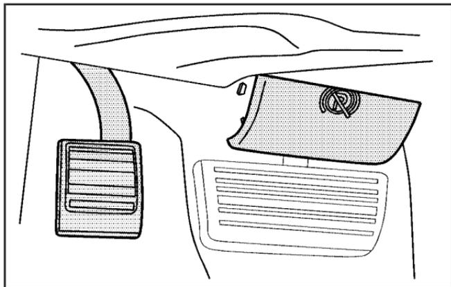
To set the parking brake, hold the regular brake pedal down with your right foot. Push down the parking brake pedal with your left foot.
