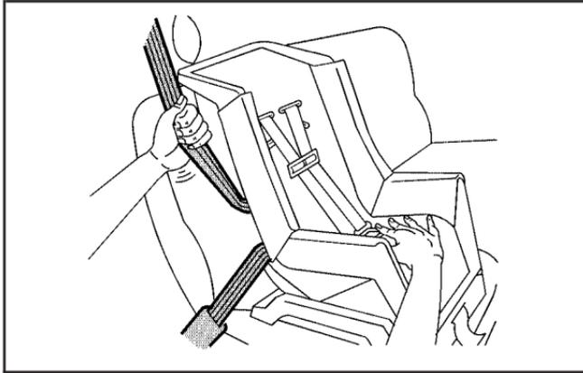
5. To tighten the belt, pull the shoulder portion of the belt to tighten the lap portion of the belt and feed the shoulder belt back into the retractor. If you are using a forward-facing child restraint, you may find it helpful to use your knee to push down on the child restraint as you tighten the belt.
