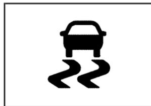
If you have the StabiliTrak® system, this light will be on or flashing, according to the description table for the StabiliTrak® system.
