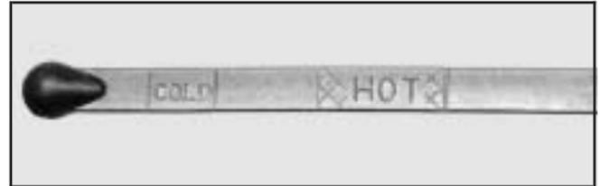
3. Check both sides of the dipstick, and read the lower level. The fluid level must be in the COLD area for a cold check or in the HOT or cross-hatched area for a hot check. Be sure to keep the dipstick pointed down to get an accurate reading.
