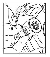
8. Put the wheel nuts back on with the rounded end of the nuts toward the wheel. Tighten each wheel nut by hand until the wheel is held against the hub.
