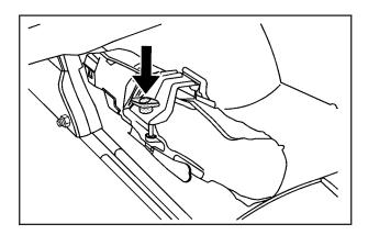
To access the equipment, remove the retaining wing bolt and lift it out of the mounting bracket.
