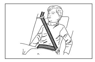
Buckle, position, and release the safety belt as described in *Rear Outside Passenger Positions on page 34*. Make sure that the shoulder belt crosses the shoulder.
