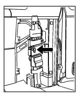
Remove the retaining wing bolt and lift it off of the mounting bracket.
