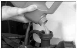
3. Fill the radiator with the proper DEX-COOL® coolant mixture, up to the base of the filler neck. See *Engine Coolant on page 308* for more information about the proper coolant mixture.
