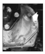
If the level is below the bottom of the filler plug hole, you may need to add some lubricant.
