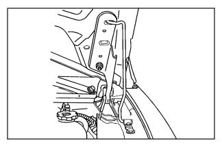
Lift the hood, release the hood prop from its retainer and put the hood prop into the slot in the hood. If your vehicle has an underhood lamp, it will automatically come on and stay on until the hood is closed.
