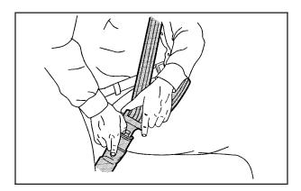
To unlatch the belt, push the button on the buckle. For outboard seating positions, when the safety belt is not in use, slide the latch plate up the safety belt webbing. The latch plate should rest on the stitching on the safety belt, near the guide loop on the side wall.
