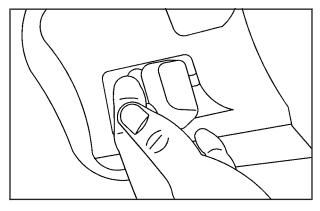
To tilt the wheel, hold the steering wheel and pull the lever. Move the steering wheel to a comfortable level, then release the lever to lock the wheel in place.
