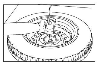
4. When the tire has been lowered, pull the tire toward you so you can reach the tire retainer and pull it up through the wheel opening.
