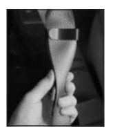
For the first row rear seat, stow the safety belt latch by attaching the clip on the safety belt latch to the trim just inside the side door.
