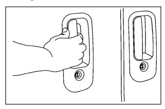
To open the sliding side door from the outside, pull the handle toward the rear of the vehicle and slide the door open.
