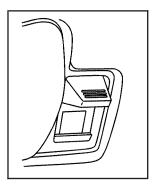
To lock the door from the inside, slide the manual lever on your door down. To unlock the door, slide the manual lever up.
