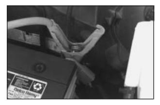
Connect the red positive (+) cable to the positive (+) terminal of the dead battery. Use a remote positive (+) terminal if the vehicle has one.
