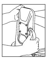
To adjust the mirrors when towing a trailer, turn the mirror by pushing the mirror head toward the front of the vehicle.
