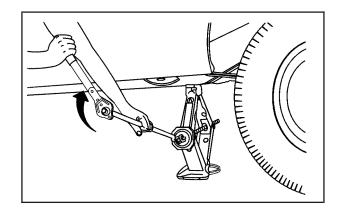
Raise the vehicle by turning the ratchet clockwise. Make sure the UP mark faces you. Raise the vehicle far enough off the ground so there is enough room for the spare tire to fit.
