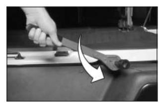
Turn the ratchet counterclockwise to lower the spare tire to the ground. If the spare tire does not lower to the ground, the secondary latch is engaged causing the tire not to lower. See Secondary Latch System on page 373.
