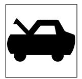
1. Pull the handle with this symbol on it. It is located in front of the driver's side door frame near the floor.
