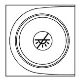
You can use the dome lamp override button, located below the exterior lamp control, to override the automatic operation of the dome lamps.
