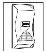
Press the bottom side of the power door lock switch to lock all the doors at once. Press the top side of the power door lock switch to unlock all the doors at once.
