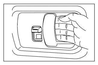
To open the front portion of a 60/40 door from the inside, pull the handle toward you and push open the door.
