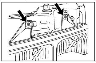
3. Remove the two pins on the top of the headlamp assembly. To remove the pins, turn the outer pin clockwise and pull it straight up. To remove the inner pin, turn it counterclockwise and pull it straight up.
