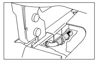
The driver's side pin has a gray cap with a black "L" marked on it.
