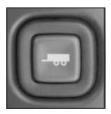
Press this button located to the right of the steering wheel on the instrument panel to turn tow/haul mode on and off.
