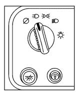
The control on the driver's side of your instrument panel operates the exterior lamps.
