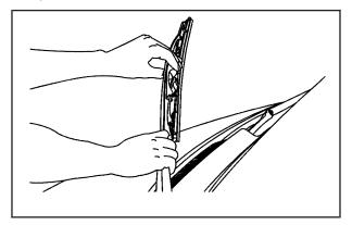
Press down on the blade assembly pivot locking tab. Pull down on the blade assembly to release it from the wiper arm hook.
