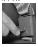
To do this, press the tip of a key into the release hole of the safety belt buckle while pulling up on the safety belt. Locate the pins. There are two pins located on the inboard sides of the rear seats. If the vehicle has floor mats, the pins will be located under a flap that has been cut into the mat.
