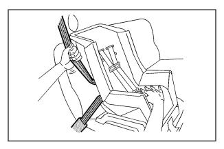
5. To tighten the belt, pull the shoulder portion of the belt to tighten the lap portion of the belt and feed the shoulder belt back into the retractor. If you are using a forward-facing child restraint, you may find it helpful to use your knee to push down on the child restraint as you tighten the belt.
