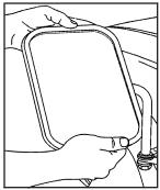
Turn the mirror head so that it swings further outboard and adjust the mirror surface as needed. Adjust the mirror by rotating it left or right. Once the mirror is adjusted to the correct position, tighten the set screw, located at the end of the arm, to hold the mirror in place. These mirrors can also be manually folded in.
