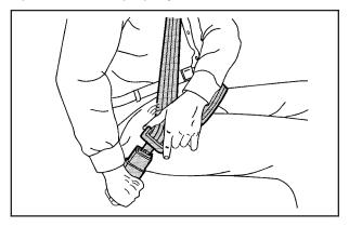
Pick up the latch plate and pull the belt across you. Do not let it get twisted. The shoulder belt may lock if you pull the belt across you very quickly. If this happens, let the belt go back slightly to unlock it. Then pull the belt across you more slowly. 2. Push the latch plate into the buckle until it clicks.
